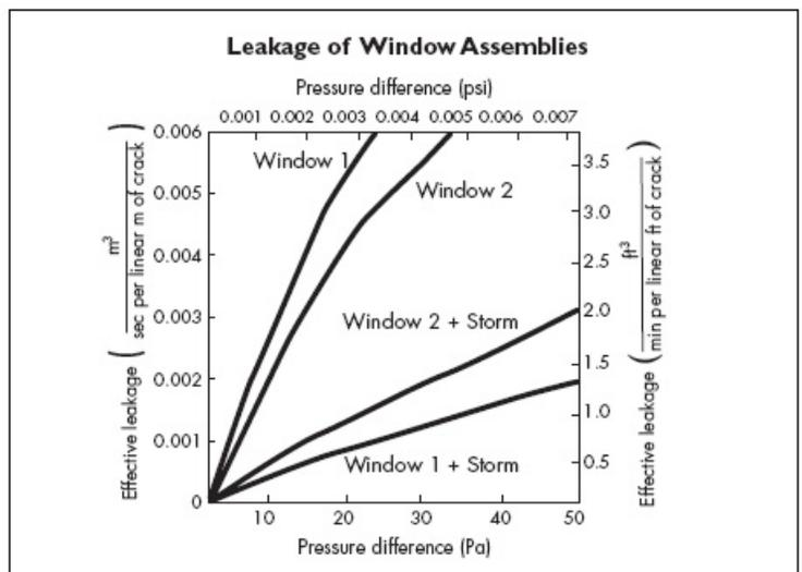
Figure 2. Air Leakage was substantially reduced after the storm windows were installed. Window One became even tighter than Window Two because of unseen leakage paths in Window Two.
